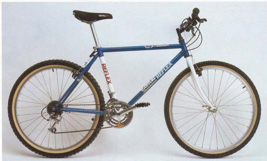
Main Frame: Painted EASTON E9 Aluminum Forks: REFLEX Designed Tange Forks Rear Triangle: Painted EASTON E9 Aluminum Lugs: Aluminum, Aerospace epoxy bond Group: Shimano 400 XL
