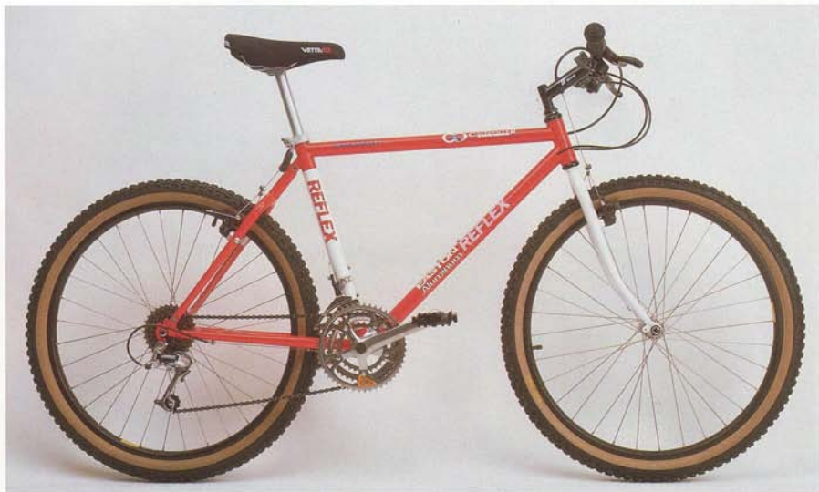
Main Frame: Painted EASTON E9 Aluminum Forks: REFLEX Designed Tange Forks Rear Triangle: Painted EASTON E9 Aluminum Lugs: Aluminum, Aerospace epoxy bond Group: Shimano 400 XL
