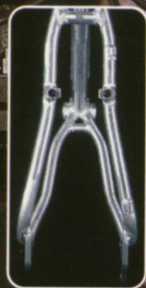
The Symmetry tail section provides powerful, flex-free braking with generous tire and mud clearance.
