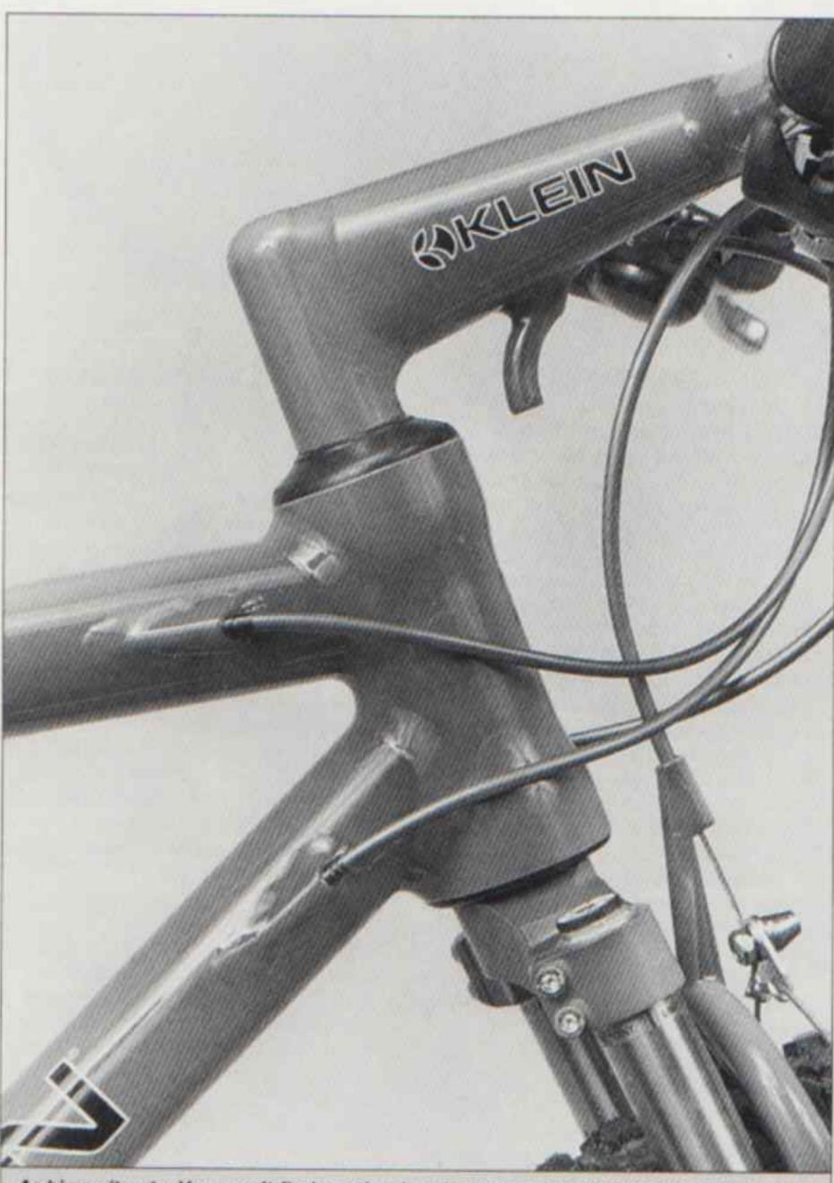
As big as it gets: You won't find another headset system on the market that is bigger than Klein's. Originally designed to accommodate the oversized aluminum steerer tube of the Klein aluminum fork, the head tube accommodates the Rock Shox steerer tube by using a steel sleeve. The Rock Shox are custom-painted to match the frame.
