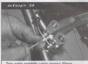
Trim extra straddle cable approx 50mm. Secure excess to brake arm with enclosed zip tie.
