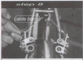
Insert end of straddle cable through hole in cable hanger. Secure adjustable cable barrel to straddle cable. Position cables as per photo and secure all bolts.
