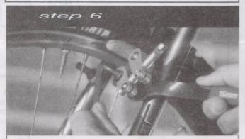
To adjust spring tension, loosen brake arm mounting bolts. Using a 15mm spanner, rotate spring tension adjuster until desired tension is achieved. Holding adjuster in place, tighten the brake mounting bolts to 6.8 N·m { 5 ft·lb } CAUTION: DO NOT OVER TIGHTEN BRAKE ARM MOUNTING BOLTS, DOING SO WILL DAMAGE THE BRAKE POSTS.
