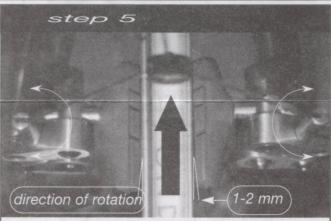
Rotate the brake holder cam. There should be a 1mm to 2mm gap at the rear of the brake pad when the front is touching the rim. Torque each pad to 6.8 N·m {5 ft·lb}
